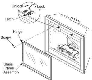
Figure 37 - Removing/Replacing Glass Door
